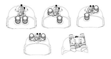
Figure 1-2. Monocular Use or Raised/Stowed Use
