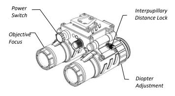
Figure 1-4. Mechanical Functions of the NORTIS-BNVS-31
