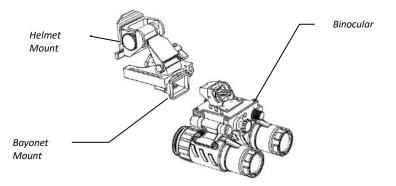
Figure 2-2. Attaching the NORTIS-BNVS-31 to Helmet Mount
