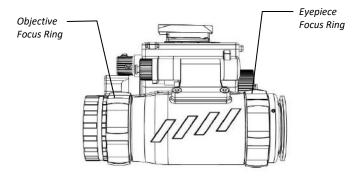
Figure 2-5. Objective Focus & Eyepiece Focus Ring
