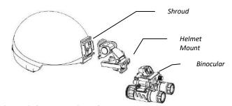
Figure 2-3. Installation of Helmet Mount to Helmet
